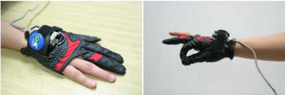
Fig. 1. The chording glove for game with the acceleration sensors to detect hand motions in space. The pinching motions generate commands for game. The thumb acts as a ground to conduct electricity to the 4 keys on the fingertips made of silicon.
