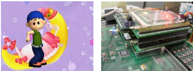
Fig. 4. A screen shot of mobile game implemented with our vertex processing unit (left) and a hardware prototype of target system using FPGA (right)
