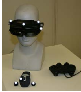
Fig. 7. The head mounted display and props used in the prototype system: upper left is an optical see-through HMD equipped with stereo circular-polarizing filters in its front, lower is a prop with buttons held by the hunter, and on the right is a game pad used by the driver. A set of infrared reflective markers were attached to the devices needed for tracking.
