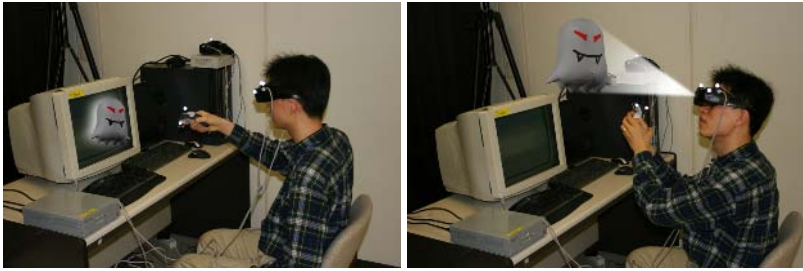
Fig. 6. A virtual object transfers from one display to another: a virtual ghost which was originally visualized on the monitor (left) popped out into the real world, visualized on the head mounted display (right)
