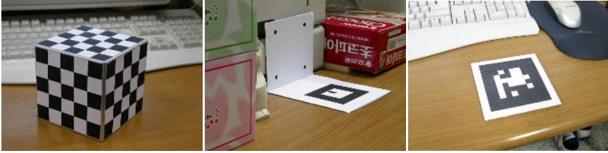
Fig. 2. Three different types of known markers: Cube , TwoSidedMarker , and ARMarker
