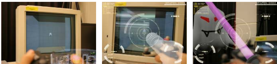
Fig. 5. Personal views of each participant: the left picture is the driver's view with a dashboard visualized on the lower right corner, the middle and the right pictures are the view of the hunter using different weapons, a proton gun and a proton saber (the pictures shown are synthesized with a photograph and a screen capture due to difficulties of taking photographs directly through head mounted displays)
