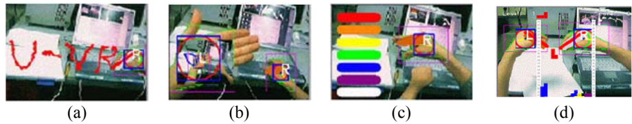
Fig. 2. (a) Memo by using a virtual pen (b) a saved image is augmented on the palm. (c) Change color of a pen (d) the user can move blocks using the finger tips in the Tetris game.
